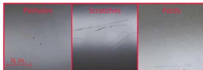
FIGURE 1. Membrane samples illustrating each of the main defect types including pinholes, scratches, and folds taken edge-lit with a compact camera
