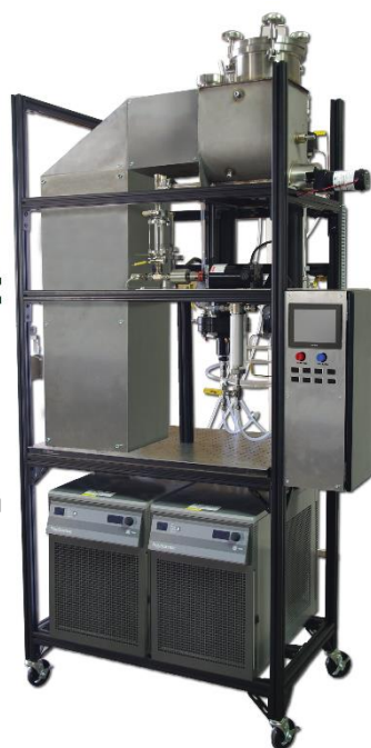
Figure 2: Mainstream's automated, continuous bench-scale pyrolysis unit.
